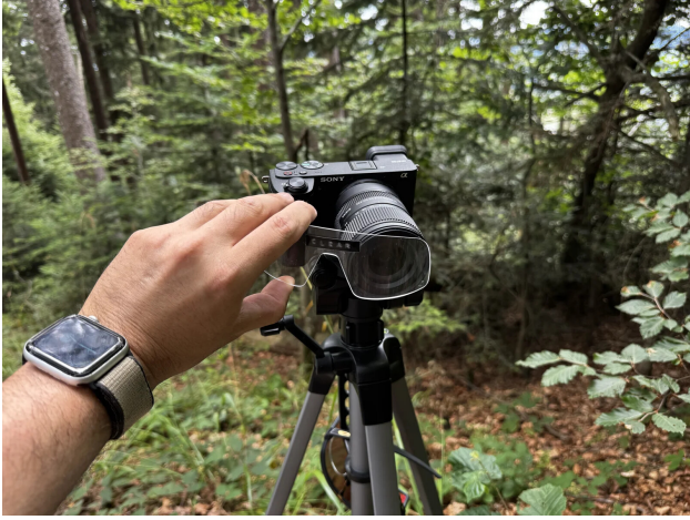
Figure 2: Field protocol. Exposure is locked once on the bare sensor; each lens is then held flat against the front element for a single frame, sixteen frames per scene in a fixed order.
